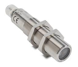
AutomationDirect photoelectric sensor, tubular, threaded, retroreflective, visible red, 1m sensing distance, complementary light-on/dark-on, PNP, teach-in button, 4-wire, 4-pin M12 quickdisconnect.
