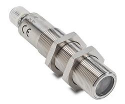
AutomationDirect photoelectric sensor, tubular, threaded, retroreflective, visible red, 1m sensing distance, complementary light-on/dark-on, NPN, teach-in button, 4-wire, 4-pin M12 quick-disconnect.
