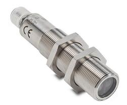
AutomationDirect photoelectric sensor, tubular, threaded, retroreflective, visible red light emission, 1m sensing distance, complementary light-on/dark-on, NPN, teach-in button, 4-wire, 4-pin M12 quick-disconnect.
