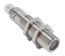
AutomationDirect photoelectric sensor, tubular, threaded, retroreflective, visible red, 1m sensing distance, selectable lighton/dark-on, PNP, teach-in button, 4-wire, 4-pin M12 quickdisconnect.
