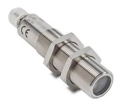
AutomationDirect photoelectric sensor, tubular, threaded, retroreflective, visible red light emission, 1m sensing distance, selectable light-on/dark-on, PNP, teach-in button, 4-wire, 4-pin M12 quick-disconnect.
