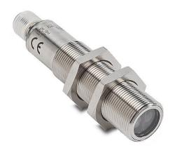
AutomationDirect photoelectric sensor, tubular, threaded, retroreflective, visible red, 1m sensing distance, selectable light-on/dark-on, NPN, teach-in button, 4-wire, 4-pin M12 quick-disconnect.
