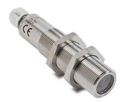
AutomationDirect photoelectric sensor, tubular, threaded, diffuse, visible red light emission, 100mm sensing distance, complementary light-on/dark-on, PNP, teach-in button, 500 Hz switching frequency, 316L stainless steel housing, 4-pin M12 quick-disconnect.
