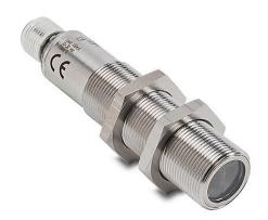
AutomationDirect photoelectric sensor, tubular, threaded, diffuse, visible red light emission, 100mm sensing distance, selectable light-on/dark-on, PNP, teach-in button, 500 Hz switching frequency, 316L stainless steel housing, 4-pin M12 quick-disconnect.
