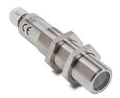
AutomationDirect photoelectric sensor, tubular, threaded, diffuse, visible red, 100mm sensing distance, selectable light-on/dark-on, NPN, teach-in button, 500 Hz switching frequency, 316L stainless steel housing, 4-pin M12 quick-disconnect.
