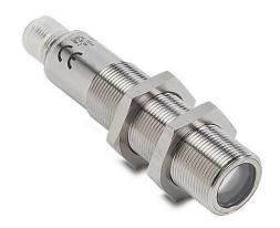
AutomationDirect photoelectric sensor, tubular, threaded, 316L stainless steel housing, through-beam receiver, 20m sensing distance, 10-30 VDC operating voltage, complementary light-on/dark-on, PNP, 4-wire, 4-pin M12 quick-disconnect.
