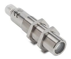
AutomationDirect photoelectric sensor, tubular, threaded, 316L stainless steel housing, through-beam receiver, 20m sensing distance, 10-30 VDC operating voltage, complementary light-on/dark-on, NPN, 4-wire, 4-pin M12 quick-disconnect.
