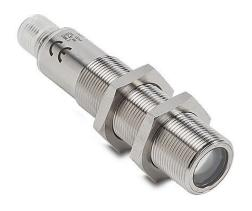
AutomationDirect photoelectric sensor, tubular, threaded, 316L stainless steel housing, through-beam receiver, 20m sensing distance, 10-30 VDC operating voltage, selectable light-on/dark-on, PNP, 4-wire, 4-pin M12 quick-disconnect.
