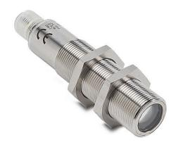
AutomationDirect photoelectric sensor, tubular, threaded, 316L stainless steel housing, through-beam emitter, infrared, 20m sensing distance, 10-30 VDC operating voltage, 3-wire, 4-pin M12 quick-disconnect.
