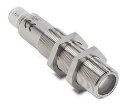
AutomationDirect photoelectric sensor, tubular, threaded, 316L stainless steel housing, through-beam emitter, infrared, 20m sensing distance, 10-30 VDC operating voltage, 2-wire, 4-pin M12 quick-disconnect.
