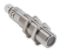
AutomationDirect photoelectric sensor, tubular, threaded, diffuse, infrared light emission, 800mm sensing distance, complementary light-on/dark-on, NPN, teach-in button, 500 Hz switching frequency, 316L stainless steel housing, 4-pin M12 quick-disconnect.
