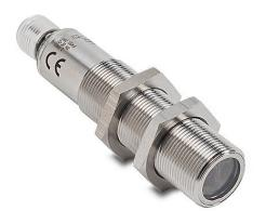
AutomationDirect photoelectric sensor, tubular, threaded, diffuse, infrared, 800mm sensing distance, complementary light-on/darkon, NPN, teach-in button, 500 Hz switching frequency, 316L stainless steel housing, 4-pin M12 quick-disconnect.
