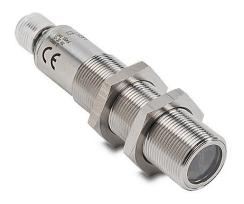
AutomationDirect photoelectric sensor, tubular, threaded, diffuse, infrared light emission, 800mm sensing distance, selectable light-on/dark-on, PNP, teach-in button, 500 Hz switching frequency, 316L stainless steel housing, 4-pin M12 quick-disconnect.
