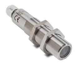
AutomationDirect photoelectric sensor, tubular, threaded, diffuse, infrared, 800mm sensing distance, selectable light-on/dark-on, NPN, teach-in button, 500 Hz switching frequency, 316L stainless steel housing, 4-pin M12 quick-disconnect.
