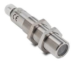
AutomationDirect photoelectric sensor, tubular, threaded, diffuse, infrared, 400mm sensing distance, complementary light-on/darkon, PNP, teach-in button, 500 Hz switching frequency, 316L stainless steel housing, 4-pin M12 quick-disconnect.
