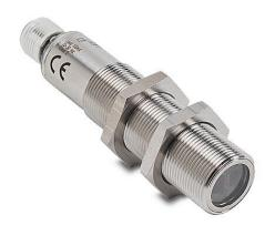
AutomationDirect photoelectric sensor, tubular, threaded, diffuse, infrared, 400mm sensing distance, complementary light-on/dark-on, NPN, teach-in button, 500 Hz switching frequency, 316L stainless steel housing, 4-pin M12 quick-disconnect.
