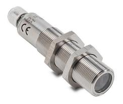
AutomationDirect photoelectric sensor, tubular, threaded, diffuse, infrared, 400mm sensing distance, selectable light-on/dark-on, PNP, teach-in button, 500 Hz switching frequency, 316L stainless steel housing, 4-pin M12 quick-disconnect.
