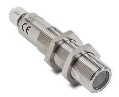
AutomationDirect photoelectric sensor, tubular, threaded, diffuse, infrared light emission, 400mm sensing distance, selectable light-on/dark-on, NPN, teach-in button, 500 Hz switching frequency, 316L stainless steel housing, 4-pin M12 quick-disconnect.
