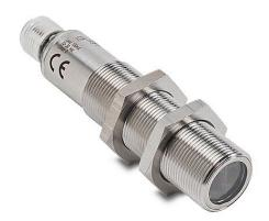
AutomationDirect photoelectric sensor, tubular, threaded, diffuse, infrared, 400mm sensing distance, selectable light-on/dark-on, NPN, teach-in button, 500 Hz switching frequency, 316L stainless steel housing, 4-pin M12 quick-disconnect.
