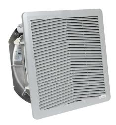
Fandis Virdis series intake fan, side mount, 436 CFM, 115 VAC operating voltage, G3 (coarse) filter mat, NEMA 12, indoor use only, 11.46 x 11.46in enclosure cutout, ANSI 61 gray.
