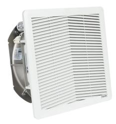
Fandis Virdis series intake fan, side mount, 436 CFM, 115 VAC operating voltage, G3 (coarse) filter mat, NEMA 12, indoor use only, 11.46 x 11.46in enclosure cutout, RAL 7035 light gray.
