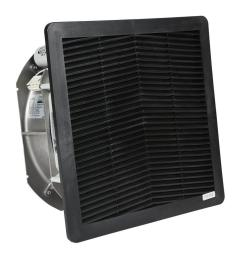
Fandis Virdis series intake fan, side mount, 436 CFM, 115 VAC operating voltage, G3 (coarse) filter mat, NEMA 3R, safe for outdoor use, 11.46 x 11.46in enclosure cutout, RAL 9005 black.
