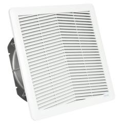
Fandis Virdis series intake fan, side mount, 297 CFM, 230 VAC operating voltage, G3 (coarse) filter mat, NEMA 12, indoor use only, 11.46 x 11.46in enclosure cutout, RAL 7035 light gray.
