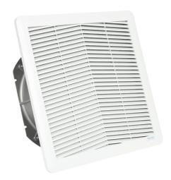
Fandis Virdis series intake fan, side mount, 297 CFM, 115 VAC operating voltage, G3 (coarse) filter mat, NEMA 12, indoor use only, 11.46 x 11.46in enclosure cutout, RAL 7035 light gray.
