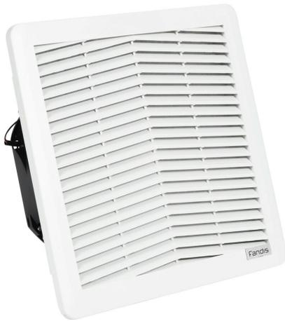
Fandis Virdis series intake fan, side mount, 175 CFM, 24 VDC operating voltage, G3 (coarse) filter mat, NEMA 12, indoor use only, 8.78 x 8.78in enclosure cutout, RAL 7035 light gray.
