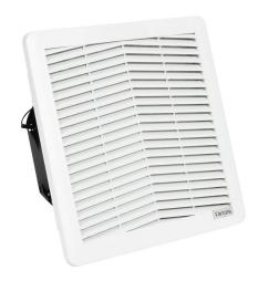
Fandis Virdis series intake fan, side mount, 175 CFM, 24 VDC operating voltage, G3 (coarse) filter mat, NEMA 12, indoor use only,  $8.78 \times 8.78$  in enclosure cutout, RAL 7035 light gray.
