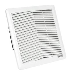
Fandis Virdis series intake fan, side mount, 159 CFM, 230 VAC operating voltage, G3 (coarse) filter mat, NEMA 12, indoor use only, 8.78 x 8.78in enclosure cutout, RAL 7035 light gray.
