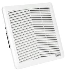
Fandis Virdis series intake fan, side mount, 155 CFM, 115 VAC operating voltage, G3 (coarse) filter mat, NEMA 12, indoor use only, 8.78 x 8.78in enclosure cutout, RAL 7035 light gray.
