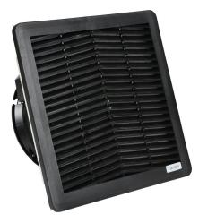
Fandis Virdis series intake fan, side mount, 112 CFM, 115 VAC operating voltage, G4 (coarse) filter mat, NEMA 3R, safe for outdoor use, 8.78 x 8.78in enclosure cutout, RAL 9005 black.
