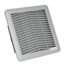
Fandis Virdis series intake fan, side mount, 59 CFM, 24 VDC operating voltage, G3 (coarse) filter mat, NEMA 12, indoor use only, 6.97 x 6.97in enclosure cutout, ANSI 61 gray.
