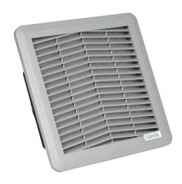
Fandis Virdis series intake fan, side mount, 59 CFM, 24 VDC operating voltage, G3 (coarse) filter mat, NEMA 12, indoor use only,  $6.97 \times 6.97$  in enclosure cutout, ANSI 61 gray.
