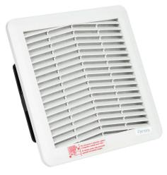
Fandis Virdis series intake fan, side mount, 65 CFM, 230 VAC operating voltage, G3 (coarse) filter mat, NEMA 12, indoor use only, 6.97 x 6.97in enclosure cutout, RAL 7035 light gray.
