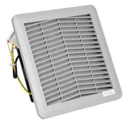
Fandis Virdis series intake fan, side mount, 65 CFM, 115 VAC operating voltage, G3 (coarse) filter mat, NEMA 12, indoor use only, 6.97 x 6.97in enclosure cutout, ANSI 61 gray.
