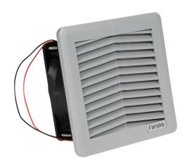
Fandis Virdis series intake fan, side mount, 27 CFM, 24 VDC operating voltage, G3 (coarse) filter mat, NEMA 12, indoor use only, 4.88 x 4.88in enclosure cutout, ANSI 61 gray.
