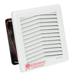
Fandis Virdis series intake fan, side mount, 27 CFM, 24 VDC operating voltage, G3 (coarse) filter mat, NEMA 12, indoor use only, 4.88 x 4.88in enclosure cutout, RAL 7035 light gray.
