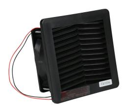
Fandis Virdis series intake fan, side mount, 21 CFM, 24 VDC operating voltage, G4 (coarse) filter mat, NEMA 3R, safe for outdoor use, 4.92 x 4.92in enclosure cutout, RAL 9005 black.
