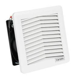
Fandis Virdis series intake fan, side mount, 29 CFM, 230 VAC operating voltage, G3 (coarse) filter mat, NEMA 12, indoor use only, 4.88 x 4.88in enclosure cutout, RAL 7035 light gray.
