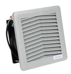
Fandis Virdis series intake fan, side mount, 29 CFM, 115 VAC operating voltage, G3 (coarse) filter mat, NEMA 12, indoor use only, 4.88 x 4.88in enclosure cutout, ANSI 61 gray.
