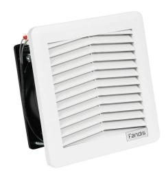
Fandis Virdis series intake fan, side mount, 29 CFM, 115 VAC operating voltage, G3 (coarse) filter mat, NEMA 12, indoor use only, 4.88 x 4.88in enclosure cutout, RAL 7035 light gray.
