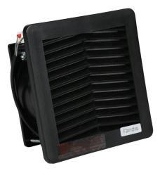
Fandis Virdis series intake fan, side mount, 23 CFM, 115 VAC operating voltage, G4 (coarse) filter mat, NEMA 3R, safe for outdoor use, 4.92 x 4.92in enclosure cutout, RAL 9005 black.
