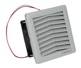
Fandis Virdis series intake fan, side mount, 9.4 CFM, 24 VDC operating voltage, G3 (coarse) filter mat, NEMA 12, indoor use only,  $3.62 \times 3.62$  in enclosure cutout, ANSI 61 gray.
