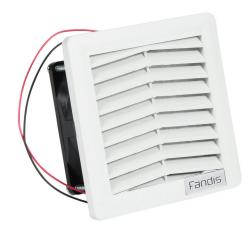
Fandis Virdis series intake fan, side mount, 9.4 CFM, 24 VDC operating voltage, G3 (coarse) filter mat, NEMA 12, indoor use only,  $3.62 \times 3.62$  in enclosure cutout, RAL 7035 light gray.
