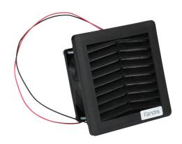
Fandis Virdis series intake fan, side mount, 9.4 CFM, 24 VDC operating voltage, G3 (coarse) filter mat, NEMA 3R, safe for outdoor use, 3.62 x 3.62in enclosure cutout, RAL 9005 black.
