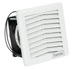
Fandis Virdis series intake fan, side mount, 8.8 CFM, 230 VAC operating voltage, G3 (coarse) filter mat, NEMA 12, indoor use only, 3.62 x 3.62in enclosure cutout, RAL 7035 light gray.
