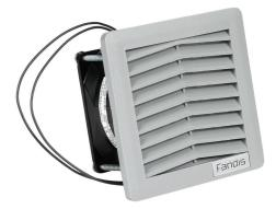
Fandis Virdis series intake fan, side mount, 8.8 CFM, 115 VAC operating voltage, G3 (coarse) filter mat, NEMA 12, indoor use only, 3.62 x 3.62in enclosure cutout, ANSI 61 gray.
