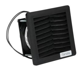
Fandis Virdis series intake fan, side mount, 8.8 CFM, 115 VAC operating voltage, G3 (coarse) filter mat, NEMA 3R, safe for outdoor use,  $3.62 \times 3.62$  in enclosure cutout, RAL 9005 black.
