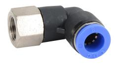
NITRA pneumatic push-to-connect fitting, elbow, rotating, thermoplastic (PBT) body, nickel-plated brass threads, (1) R1/8 female BSPT to (1) 5/16in (8mm) push-to-connect. Package of 5.
