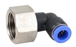
NITRA pneumatic push-to-connect fitting, elbow, rotating, thermoplastic (PBT) body, nickel-plated brass threads, (1) R1/2 female BSPT to (1) 5/16in (8mm) push-to-connect. Package of 5.
