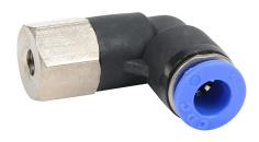
NITRA pneumatic push-to-connect fitting, elbow, rotating, thermoplastic (PBT) body, nickel-plated brass threads, (1) M5  $\times$  0.8 female ISO to (1) 6mm push-to-connect. Package of 5.
