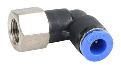
NITRA pneumatic push-to-connect fitting, elbow, rotating, thermoplastic (PBT) body, nickel-plated brass threads, (1) R1/8 female BSPT to (1) 6mm push-to-connect. Package of 5.
