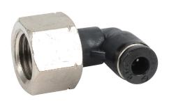
NITRA pneumatic push-to-connect fitting, elbow, rotating, thermoplastic (PBT) body, nickel-plated brass threads, (1) 1/4in female NPT to (1) 5/32in (4mm) push-to-connect. Package of 5.
