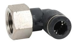
NITRA pneumatic push-to-connect fitting, elbow, rotating, thermoplastic (PBT) body, nickel-plated brass threads, (1) 3/8in female NPT to (1) 3/8in push-to-connect. Package of 5.
